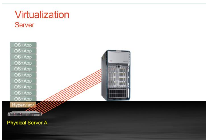
4.19. Single physical server hosting multiple VMs
